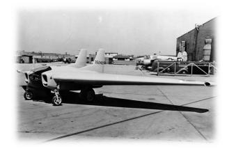
Instead of relying on heavy guns, the XP-79 would collide with other aircraft, using its strong wings to tear through the wings or fuselages of enemy bombers.
